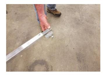
Remove vertical locking pin to rotate the top plate. Insert pin to lock top plate in place. 19
