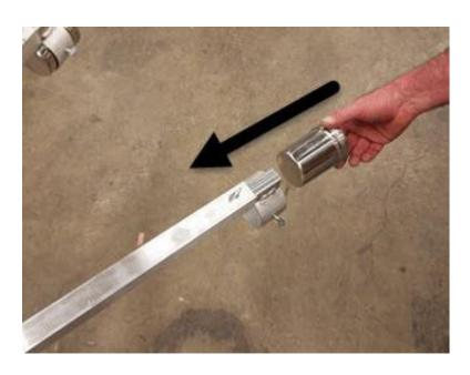
Place ID Tab under the top plate at the base of each arm. Loosen bolts to slide under then tighten again.
