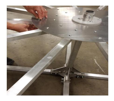
Insert a short arm into each long arm and secure in place with a thumbscrew
